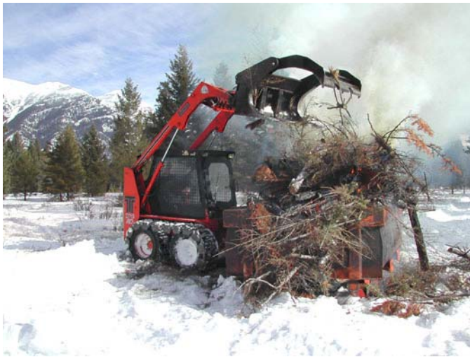
Figure 2: Burning in a sloop is a low-impact way to dispose of the small trees cut during slashing. Sloop-burning produces less smoke and less soil damage than pile-burning slash on the ground. Sloops used in the Trench restoration program are made in the East Kootenay from ore cars once used underground in Kimberley's Sullivan Mine (photos and text from Rocky Mountain Trench Committee 2006).
